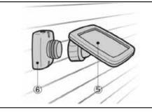
2.Drill two holes on the wall based in the holes in the panel base, then insert in the panel base, then insert the bulged tubes into the holes. Finally fix the panel base on the wall by screws.
